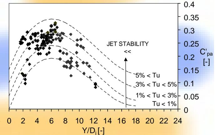
$$C_{pa} = 38.4 \cdot (1 - \alpha_i) \cdot \left(\frac{D_j}{Y}\right)^2 \quad \text{for } Y/D_j > 4-6$$
